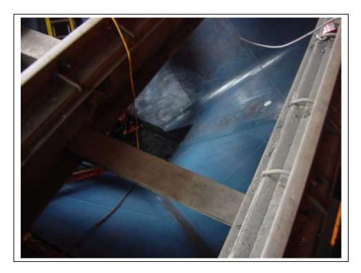
Time has now come for the replacement of the TIVAR® 88-2 liner. While still functioning well, areas around the discharge are worn. Due to the success of the liner, AEP has opted to have the SystemTIVAR® Engineering Group install a new TIVAR 88-2 liner. The liner system will be installed in May 2010 and is ready for another eight million tons.
