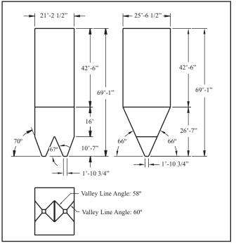
Figure 6. Unit 8 bunker dimensional layout
