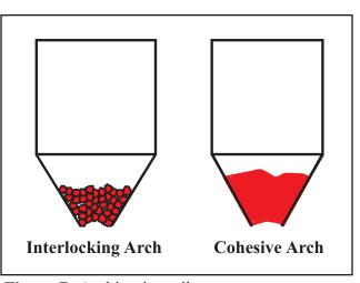
**Figure B.** Arching in a silo – interlocking or cohesive
