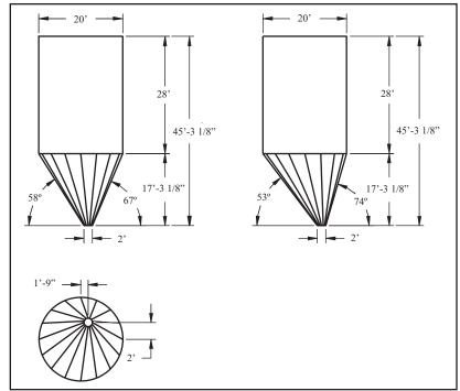
Figure 4. Dimensional layout of original Unit 5 bunker
