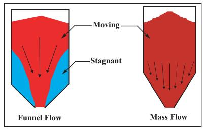
Figure C. Funnel flow and mass flow
