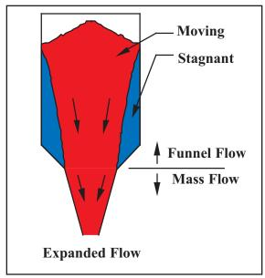
Figure D. Expanded flow pattern in a silo
