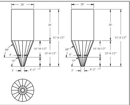
**Figure 5.** Unit 5 bunker modification with symmetric two-stage conical hopper.
