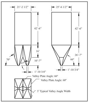
Figure 8. Dimensional layout for Unit 8 modification
