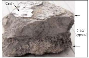
Figure 1. Typical gunite coating portion
